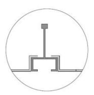
Flat leveled bedding panel lay in groove carrier
