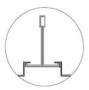
Lower leveled bedding panel lay in flat carrier
